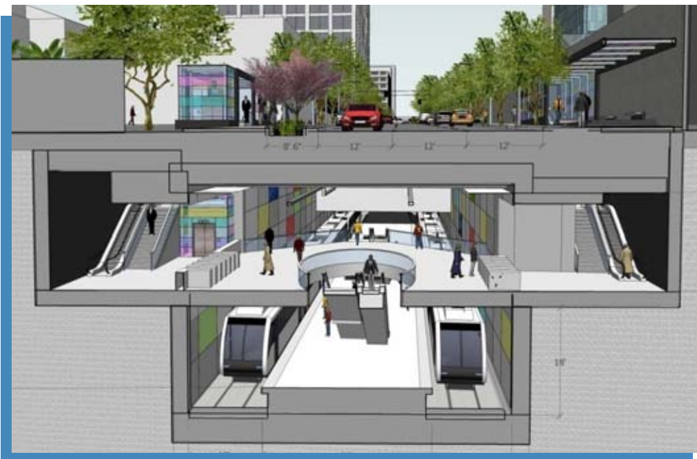
Figure 2-6. Typical Underground Station
