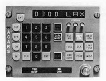
A new development in communications for the airlines will automatically provide vital flight information to ground personnel over an ARINC VHF network at a cost, speed, and accuracy not possible through present manual/voice communications. ACARS is an addressable digital data link system which permits routing of messages to and from a particular aircraft.
