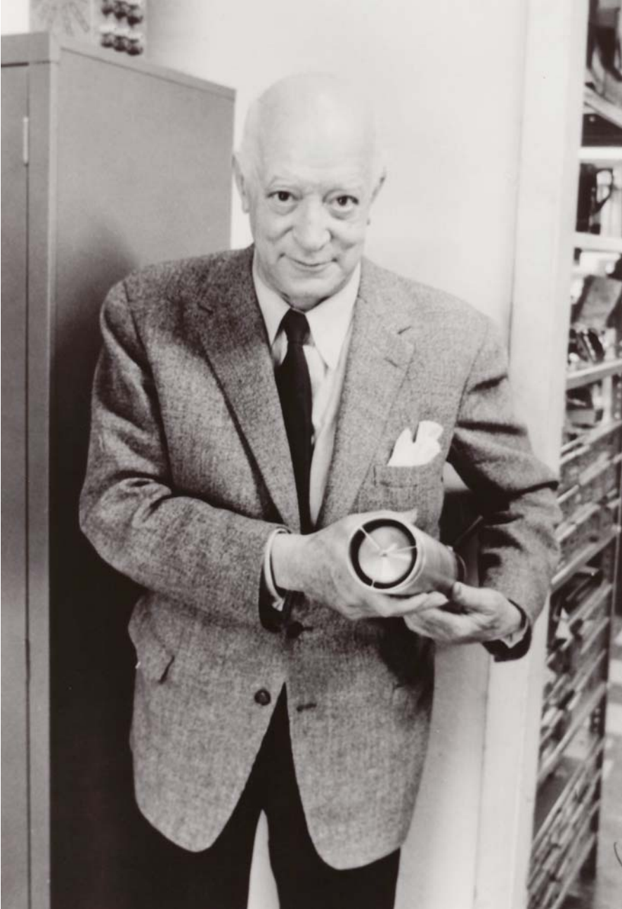
Dr Henri-Marie Coanda holding a test model of a shrouded Coanda Effect internal nozzle he designed for underwater propulsion using steam as the primary fluid. Device was tested at Huyck Research Laboratories in Stamford, Connecticut, in 1963 , but no interest was shown by the United States Navy in spite of highly successful water tunnel tests at Huyck.
