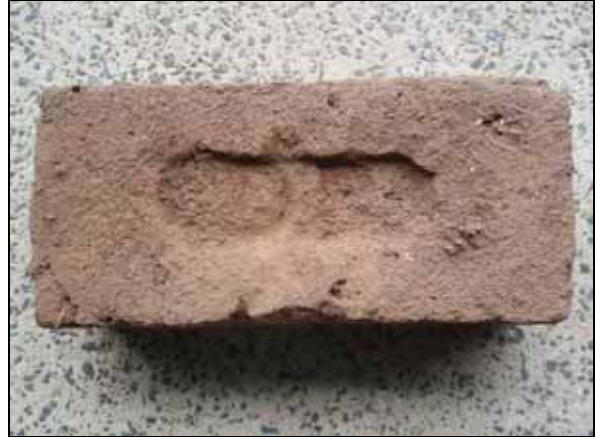
Figure 8.104: G2B H42 – An example of a 'David Berry brick', of which many have been found on site. Note 'D B' impressed within frog
