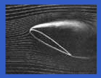
Apparently the glass got a small accidental leak providing small air bubbles acting as continuous tracers (1897).
