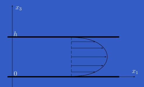
$x_1, x_3$ -section of the Hele-Shaw cell. Suppose that the flow is parallel and slow:
