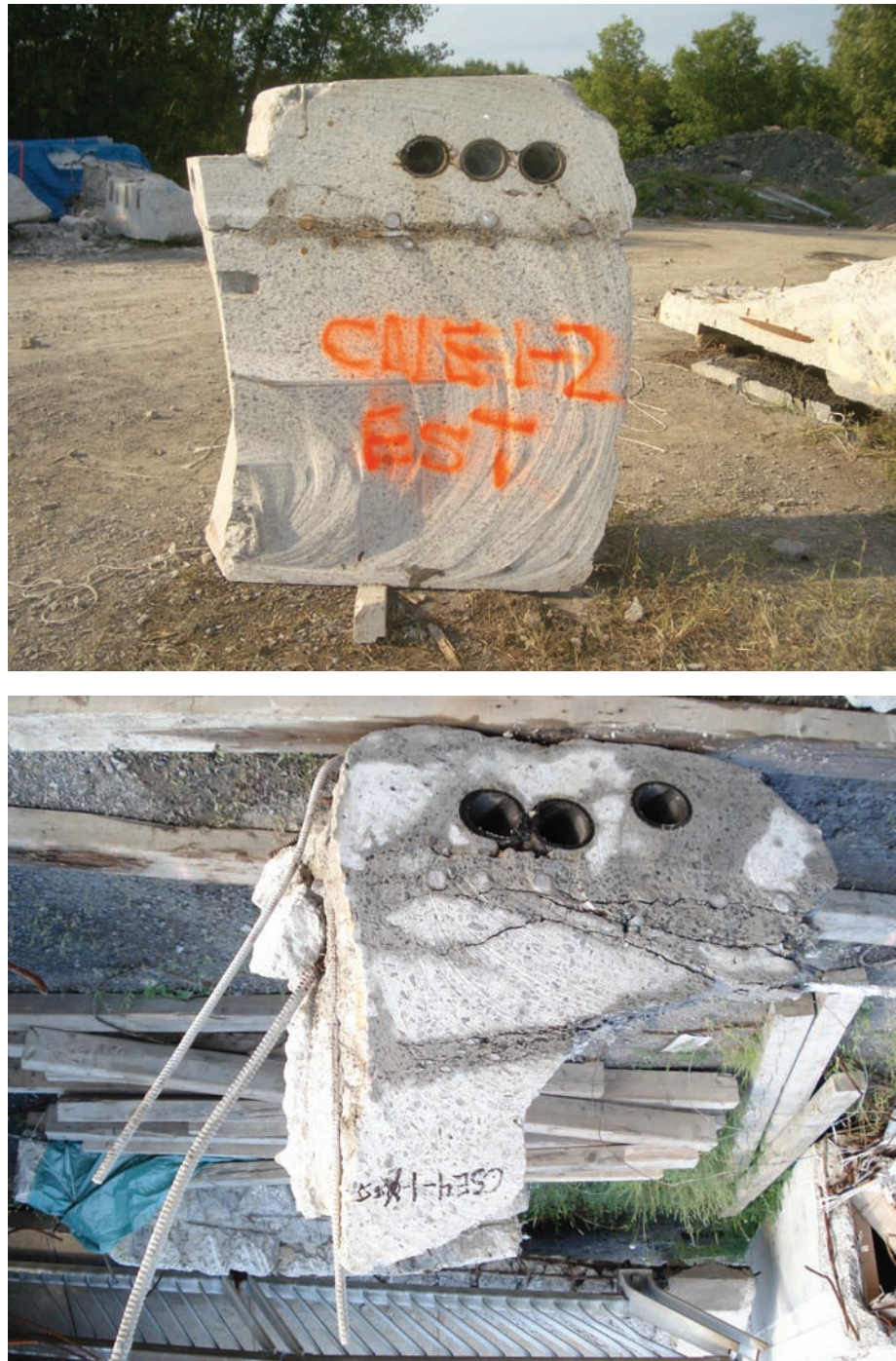
Figure 5.8 Transverse partial cuts of the east abutment performed during the additional dissection operations of August 2007 showing the northeast corner (top) and southeast corner (bottom) 105
