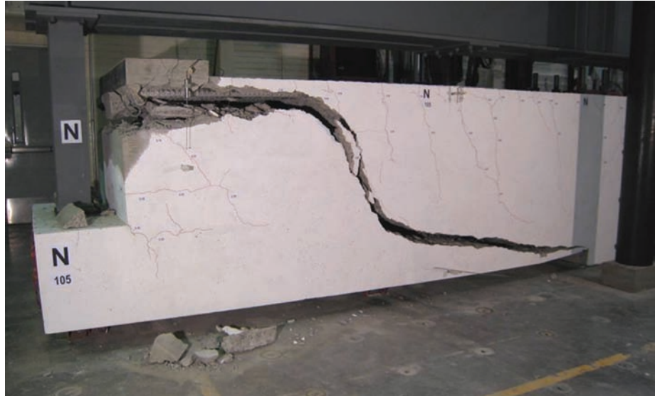
Figure 5.7 Failure of the “as-built” cantilever during the laboratory loading tests at McGill University 90
