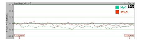
Figure 12: This figure is used to further illustrate the "strait cut" exhibited by the LAME encoder at high frequencies.
