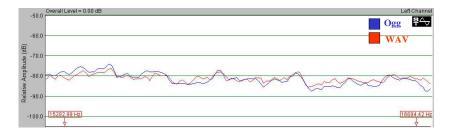
Figure 11: The important thing to notice here is that Ogg remains "brilliant" at high frequencies. It is almost identical to the original wave file wave form.
