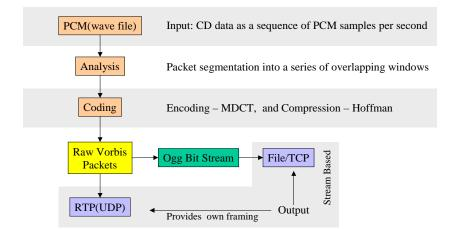
Figure 2: The complete process of input, analysis, encoding, and output.
