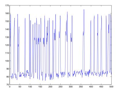
Figure 13: frame number versus bitrate for the file macy.ogg
