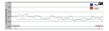
Figure 10: A closer look at what happens at high frequency ranges. Ogg has a better handel on the frequency ranges above the 15kHz mark when compared to Mp3.
