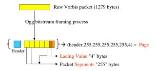
Figure 3: The raw Vorbis packets are logically segmented into a set of segments of length 255 bytes. The last segment is the *lacing value* which must be < 255 and is used as a recapture sequence marker.
