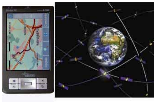
Figure 7 - A palm-top with built-in GNSS receiver. This daily life device requires a 30 satellite constellation with associated highly available ground segment
