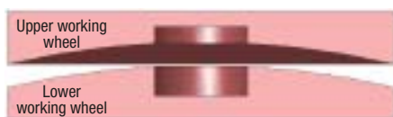
Fig 2 Possible wear pattern on tools for flat honing
