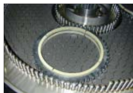
Fig 8 Dressing and sharpening ring in use
