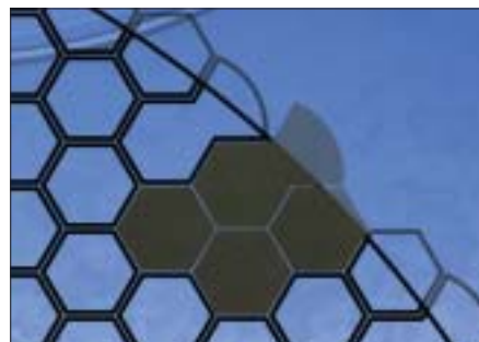
Fig 6 Technical design to stabilise the edge zone of a CBN/diamond wheel for flat honing (schematic) – goldfish pellets
