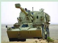
In a continuing drive to improve its acknowledged lead in tubed artillery systems, Denel shattered all previous artillery records by firing 75km earlier this year. This range improvement was achieved on 11 April 2006 with the latest G6-52L, Denel's extended range version of its renowned G6 self-propelled artillery system. It fired V-LAP projectiles which use both base-bleed and rocket-assist technology to extend the range.
