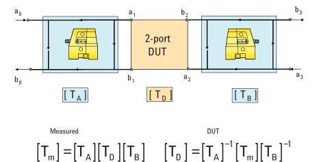
Figure 17. Principle #5: De-embed fixtures from measurements using T-parameter matrices
