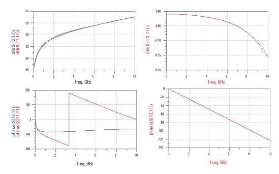
Figure 36. S-parameter of the SMA launch with a zero length transmission line segment
