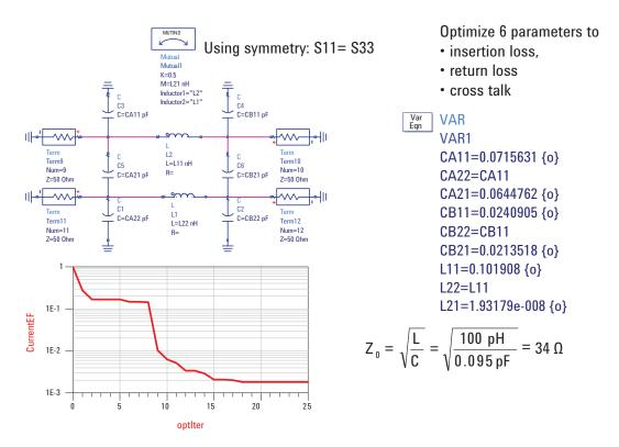
Figure 50. Building a simple C-L-C model of the vias
