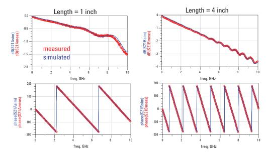
Figure 33. Insertion loss: measured and modeled
