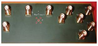
Back side of the board with SMA connector launches
