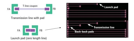
Figure 40. FPGA test fixture de-embedding
