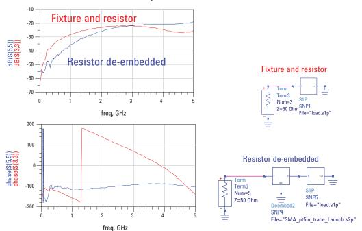
Figure 38. De-embedded termination
