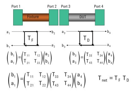
Figure 14. Cascading T-parameters
