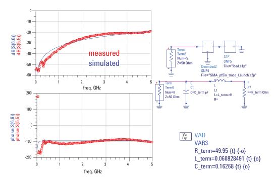
Figure 39. Modeling the terminating resistor
