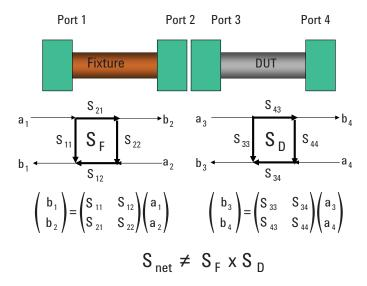
Figure 11. Principle #4: Cascading signal flow diagrams
