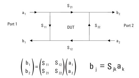
Figure 10. Principle #3: Signal flow diagrams
