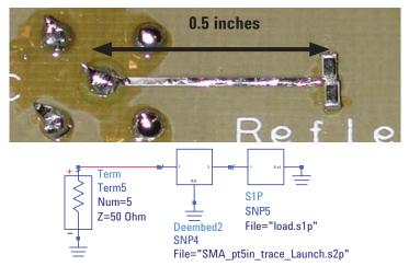
Figure 37. Model for a 50 Ohm load
