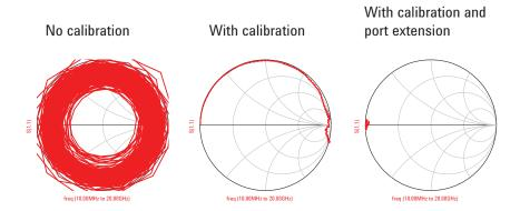
Figure 4. Impact of calibration on a short at the end of a 1 m precision cable
