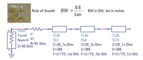
Figure 31. Building a model for an SMA launch
