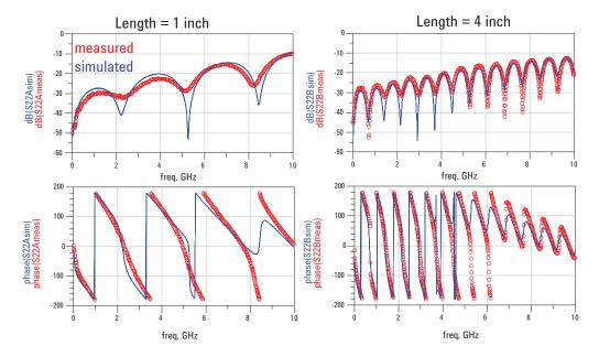
Figure 34. Return loss: measured and modeled
