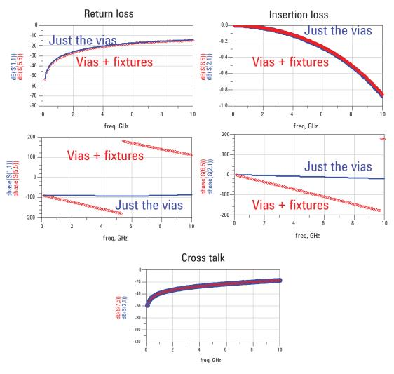
Figure 49. Impact of de-embedding: de-embedding is critical for accurate phase simulation
