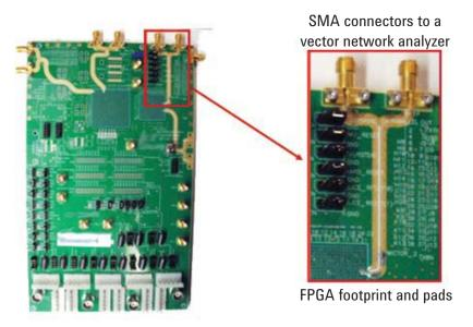
Figure 1. De-embedding: removing fixture effects from a measurement.
