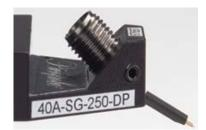
Thru connection, with the microprobe to be measured inserted, using unknown thru calibration
