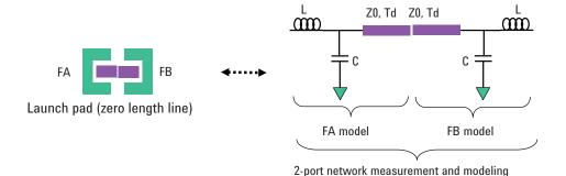
Figure 41. FPGA test fixture de-embedding
