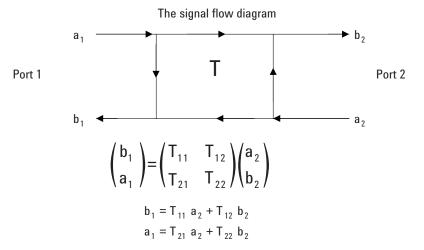
Figure 12. The transfer-parameter or T-parameter matrix
