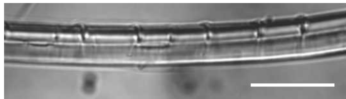
Figure 3.13. Optical micrograph of an elementary flax fibre in a loop with local fibre thickening at the compression side of the fibre. Scale bar indicates 50 \mu\text{m} .
