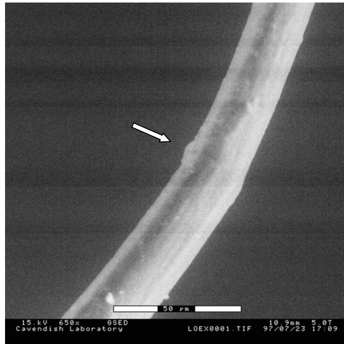
Figure 3.19. ESEM micrograph of an elementary flax fibre which has just started to developed a kink band, marked by the arrow. Scale bar indicates 50 µm.
