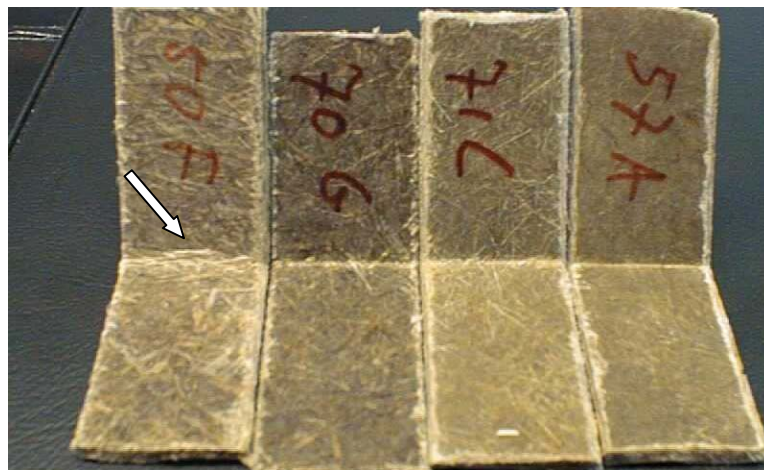
Figure 5.13. Photograph of the blow side of Charpy impacted flax/PP composites; from left to right: scutched flax/PP, scutched flax/PP/MAPP, hackled flax/PP and hackled flax/PP/MAPP. The arrow indicates where the scutched fibres buckle out in the scutched flax/PP composite.
