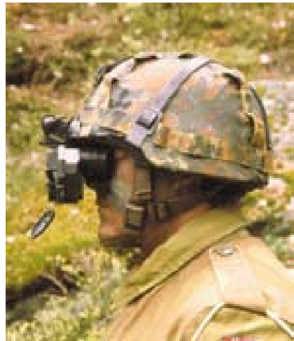
Simrad's night vision goggles can be helmet of head mounted.(PHOTO: Simrad)
