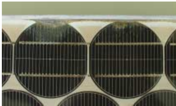
Figure 10: Delamination affecting cells nr. 5 and 6 of the ASI16-2300 module A005.
