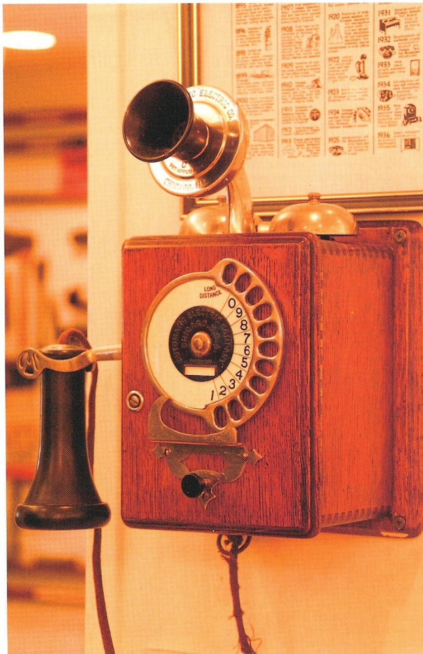
This Strowger Automatic Dial System phone was the latest and greatest of its time.
