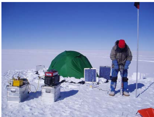
Research partner Geoff Somers drills the hole for the density measurement instruments. Photo: Liz Morris
