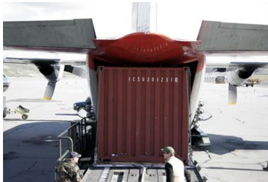
A DISC container just fits the C-130 cargo hold. Ben Toth in foreground. Photo: Ed Stockard
