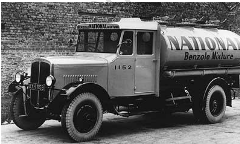
Speedy normal control petrol tanker looks rather car-like forward of the cargo tank.
