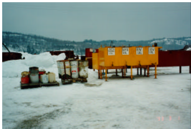
Collection and storage of waste oils prior to shipping by waste oil handler.
