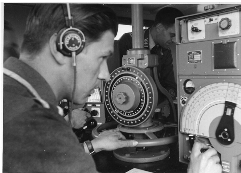
Interior: Operator at EP2a RX (75 kHz - 3.3 MHz).
