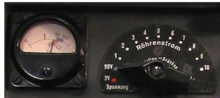
Built-in test meter for battery voltages & tube anode currents courtesy LA6NCA
