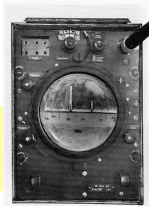
VHF spectrum analyzer W.Anz.g2 (FuMB 9) for 146-254 MHz. Push-pull RF amp and mixer with acorn tubes. RBW: \pm 300 kHz. Sensitivity: 300 \mu\text{V} for 10 dB S/N.
