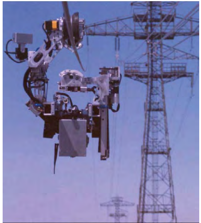
Figure 9: A successful test on an energized 315 kV circuit.
