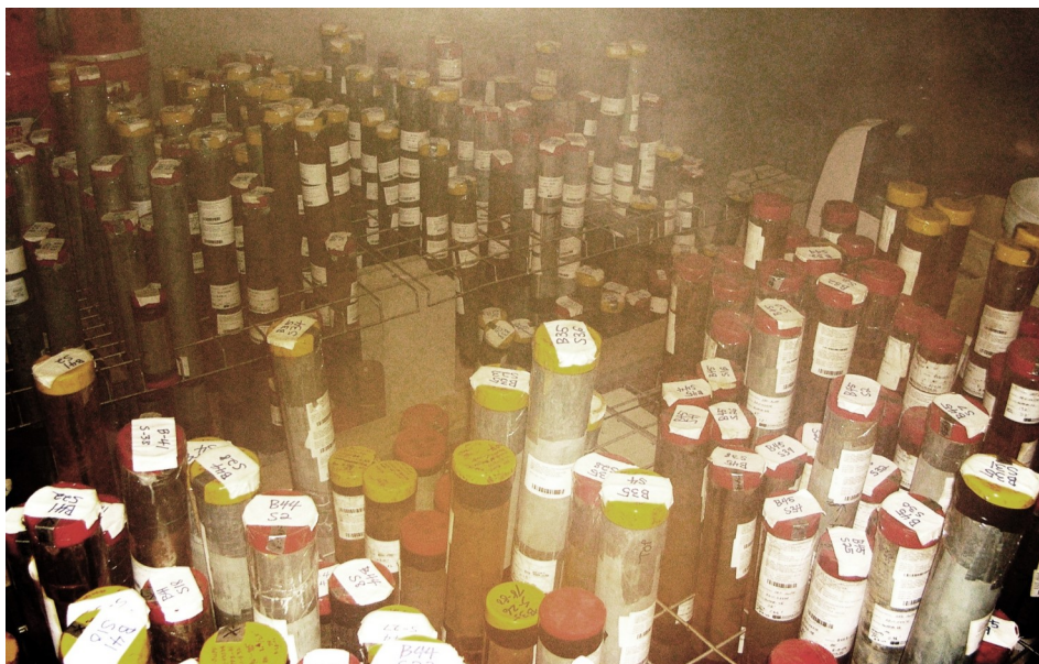
Shelby tube samples in the 100%-relative-humidity chamber
