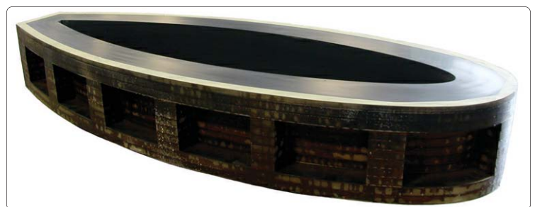
Female mold for lay-up of streamlined carbon fairings for US Navy vessels' sensors.
