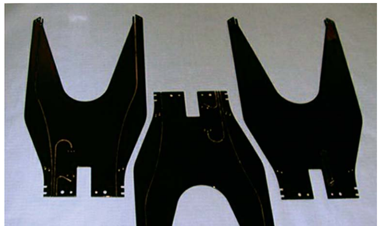
Robotic production-line wafer handling relies on GMT's carbon effectors.
