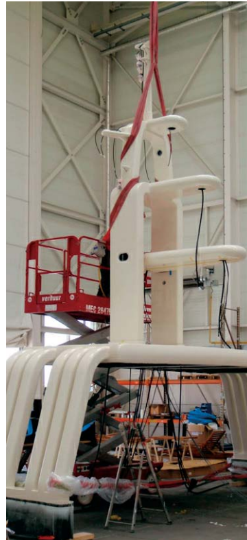
Calliope's electronics arch awaits installation.
