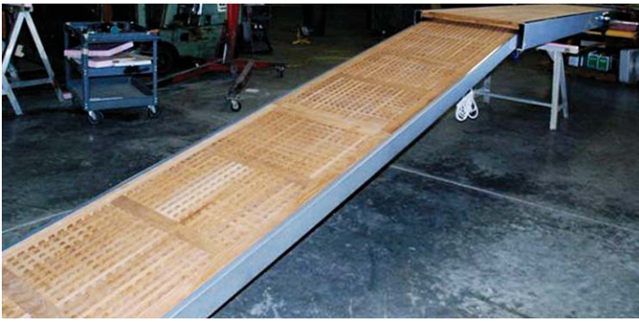
Dock in deployed mode, with carbon and teak ramp angled down to land.
