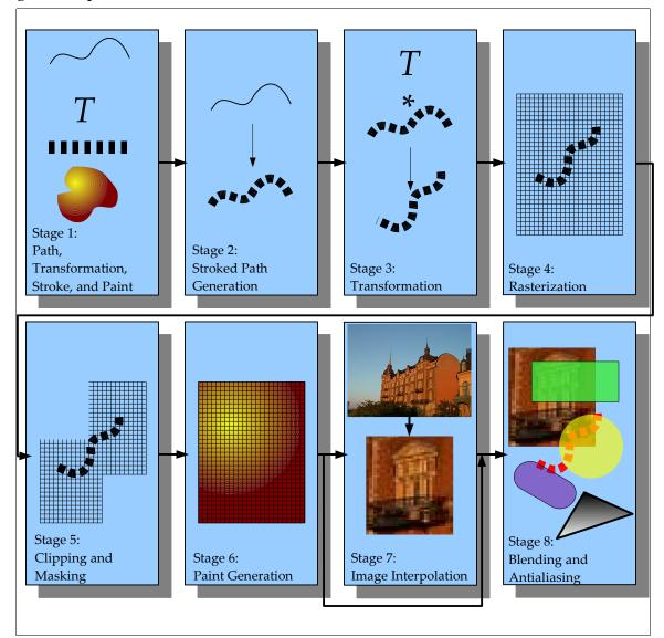
Figure 1: The OpenVG Pipeline
