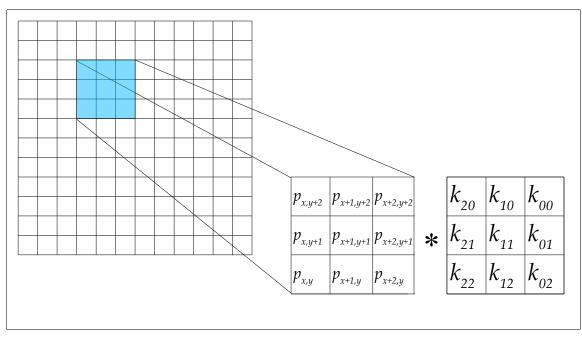
Figure 23: Convolution With a Flipped Kernel
