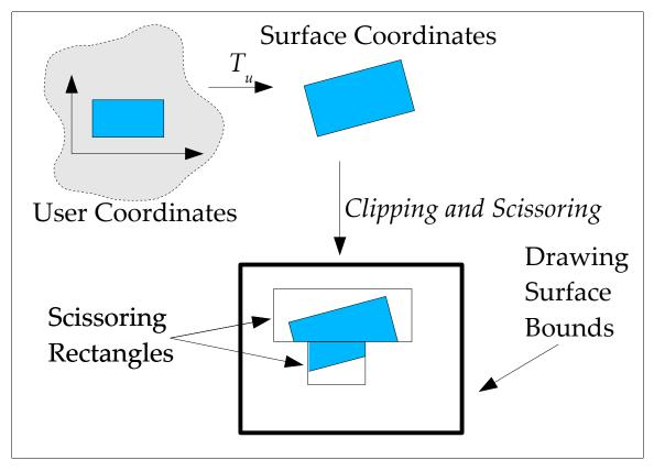
Figure 3: Coordinates, Transformation, Clipping, and Scissoring
