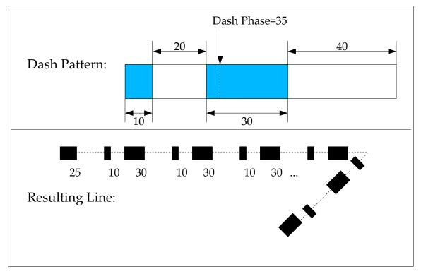
Figure 17: Dash Pattern and Phase Example
