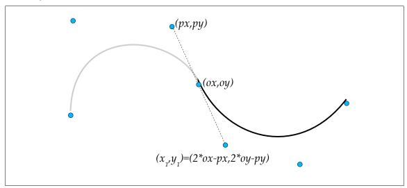
Figure 4: Smooth Curve Construction
