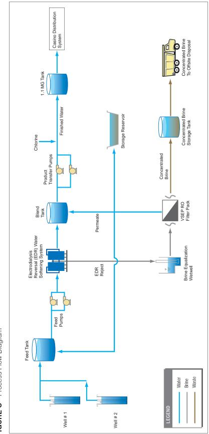
FIGURE C-Process Flow Diagram
