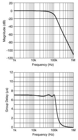
Figure 4. Linear Phase Filter
