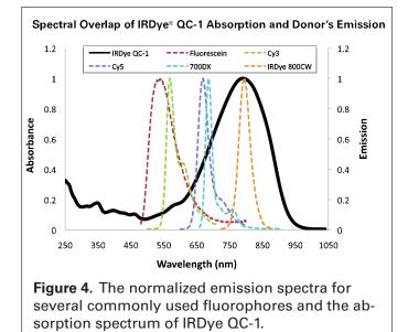
The broad absorption peak of IRDye QC-1 spans the entire visible region and into the near infrared region of the spectrum, with a maximum at 737 nm and a shoulder at 815 nm (Figure 4). The quenching range
