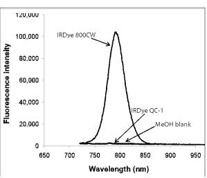
**Figure 5.** Fluorescence spectra of IRDye 800CW and IRDye QC-1 in methanol (each at 0.01 OD absorbance at 700 nm) following excitation by 700 nm light.
