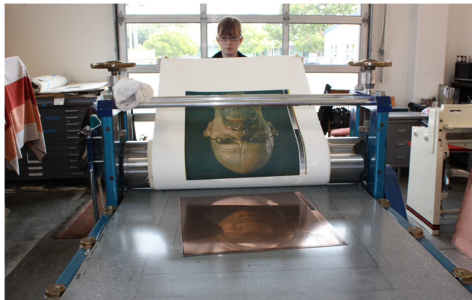
Michelle Morgan pulls a proof of the color direct-to-plate photogravure at Paulson Press. A separate plate was etched, inked, registered and printed for each color.
