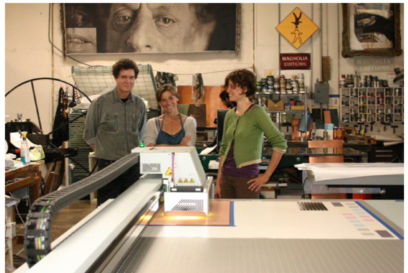
Donald Farnsworth, Renee Bott, and Tallulah Terry at Magnolia Editions while the UV inkjet printer lays down a mask on a copper plate. The treaded gantry along which the print heads move in three dimensions extends into the foreground at left.
