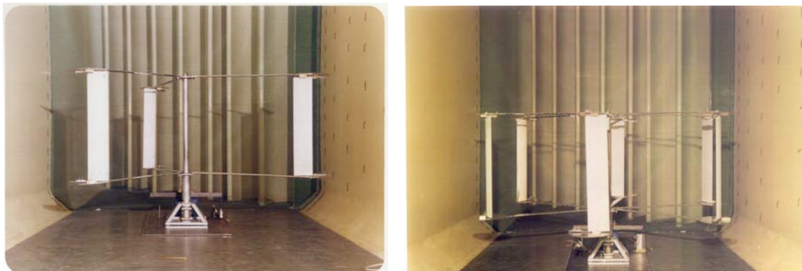
Fig. II. Model of Kobold turbine installed in the wind-tunnel belonging to Dipartimento di Progettazione Aeronautica of University of Naples (3 blades, left; 6 blades, right)
