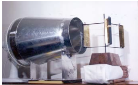
Fig. I – First small model of turbine (Panemone type) for tests in water tank of Dept. of Naval Architecture of University of Naples
