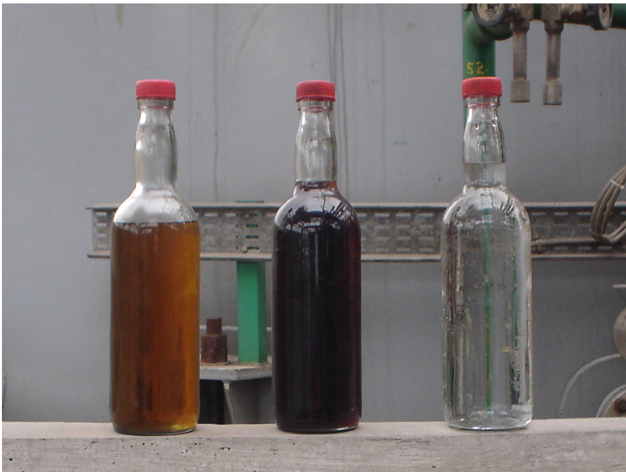
Figure 4. Sulfidic spent caustic (left), main spent caustic (center), and oxidized effluent (right)
