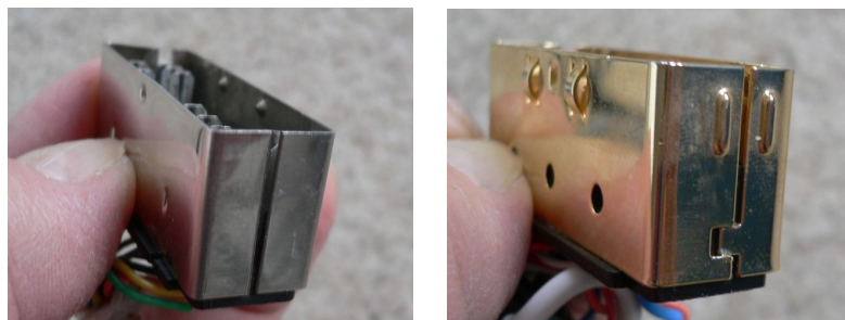
Fig. 3 – the metal shield of a standard SCART plug (left) and an example of shaping to improve robustness (right)
