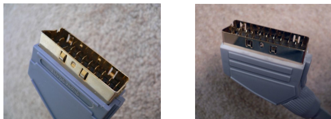
Fig. 6 - Examples of improved locking mechanisms in the shield of a secure SCART
