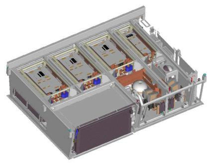
The converter modules are liquid cooled where the coolant is a mixture of water and an anti-freeze agent. The coolant is cooled in a liquid to air heat exchanger placed in the converter box. In order to avoid internal hot spots the converter box is also equipped with an internal fan.
