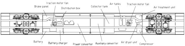
The Mc and the M cars have the same electrical system structure and equipment except for the additional equipment in the end car for the driver's cab and ATP antennas. All four axles are driven in the motorized cars.
