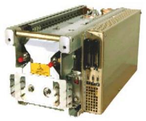
the traction converter. The auxiliary converter converts the DC voltage to a three-phase voltage. A filter reduces the electric harmonics from the converter output. A transformer isolates the high voltage converter output from the  $3 \times 400$  V, 50 Hz network.
