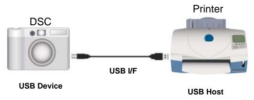
Fig. 2 Connection of PictBridge compliant devices
