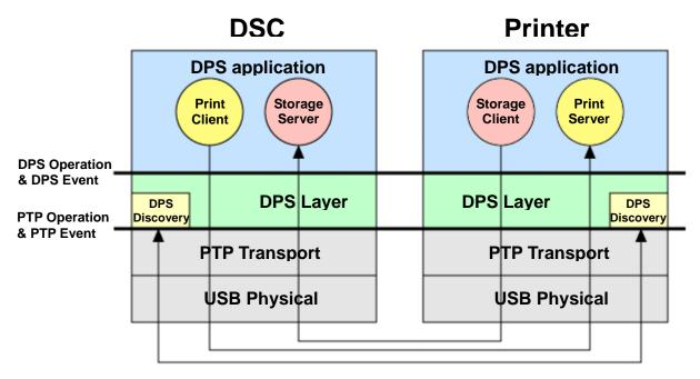
Fig. 3 communication protocol architecture
