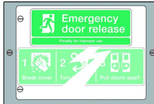
Cover in place: sign 1 on the cover and sign two visible through the cover
