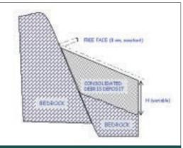
Fig. 12. Schematic section of the reactivated fault zone at Costa, used for modeling the possible causes of observed slip.
