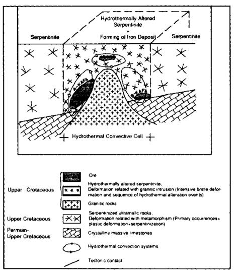
Fig. 3- Schematized formation model of Divrigi A- and B- Kafa iron deposits (non scaled).
