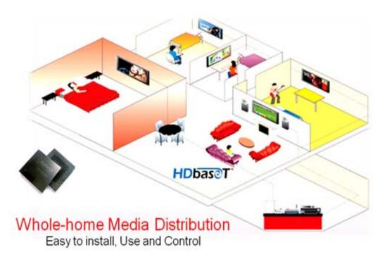
What are the cable-length advantages offered by HDBaseT? HDBaseT can support 100m/328f at the minimum, enabling much longer distances than other alternatives. HDBaseT technology seamlessly travels distances which would otherwise be extremely costly when using other available cables. Not only is the added reach a cost-saving factor, but HDBaseT technology cuts down the number of cables required in all.
