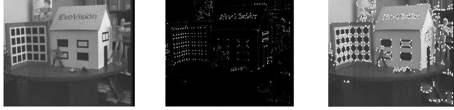
Figure 1: A look at interest point detection: left, an input image I ; middle, interest image I^* ; right, detected points after non-maximum suppression and thresholding superimposed on I . Interest points were detected with the K_{IPGP2} operator.
