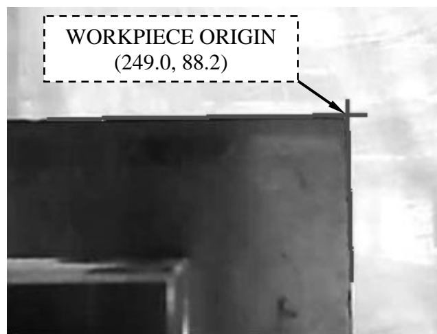
Figure 9: Determined coordinates of the zero point.
