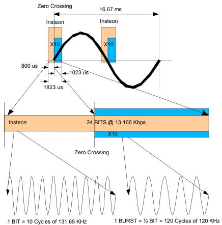
The top of the figure shows a single powerline cycle, which possesses two zero crossings. An INSTEON packet is shown at each zero crossing. INSTEON packets begin 800 microseconds before a zero crossing and last until 1023 microseconds after the zero crossing.
