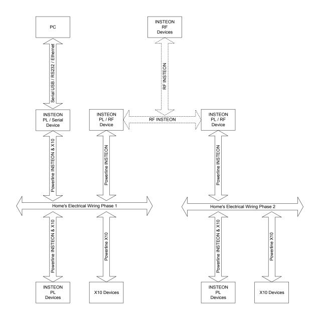
Electrical power is most commonly distributed to homes in North America as splitphase 220-volt alternating current (220 VAC). At the main electrical junction box to the home, the single three-wire 220 VAC powerline is split into a pair of two-wire
