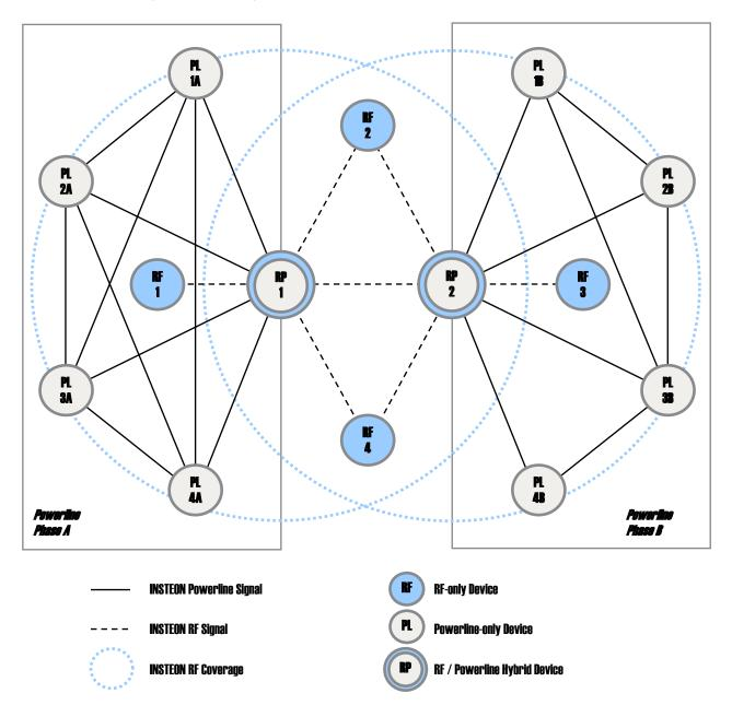
Every INSTEON device is capable of repeating<sup>1</sup> INSTEON messages. They will do this automatically as soon as they are powered up—they do not need to be specially installed using some network setup procedure. Adding more devices increases the number of available pathways for messages to travel. This *path diversity* results in a higher probability that a message will arrive at its intended destination, so the more devices in an INSTEON network, the better.
