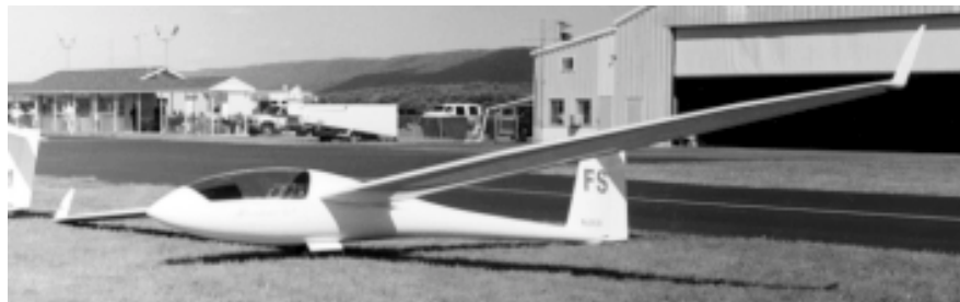
Once a rarity on sailplanes, winglets have become standard equipment on the aircraft.
