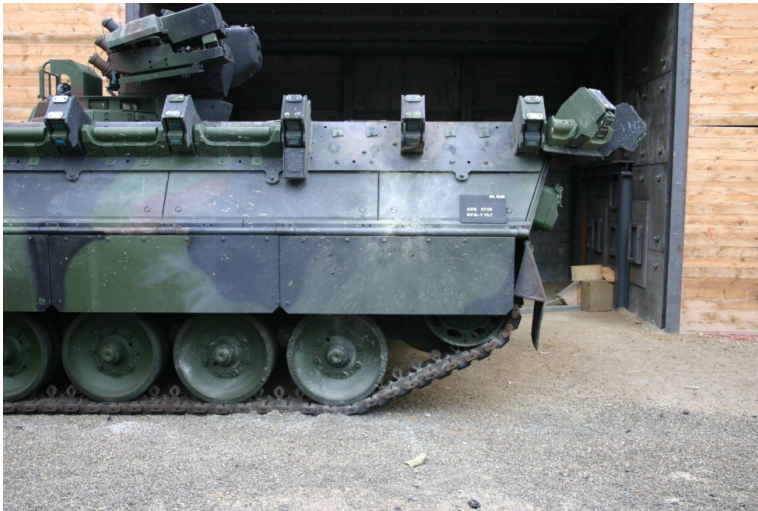
IFV Marder with AMAP-ADS after successful defeat of 2 RPG-7
