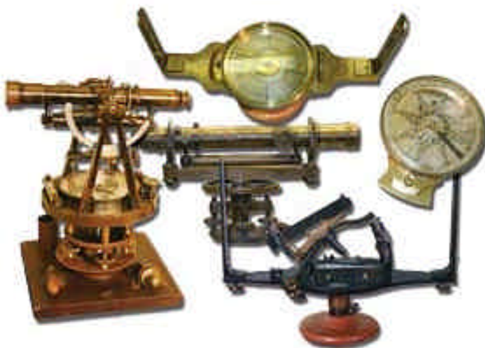
Clockwise from top: vernier compass (Thomas Whitney, Philadelphia, Pa., 1820), Rittenhouse compass (Benjamin Rittenhouse, Philadelphia, Pa., ca. 1780), William Austin Burt solar compass (William J. Young, Philadelphia, Pa., ca. 1840), transit (L. Beckmann Co., Toledo, Ohio, ca. 1885), architect's level (L. Beckmann Co., Toledo, Ohio, ca. 1911). 18
