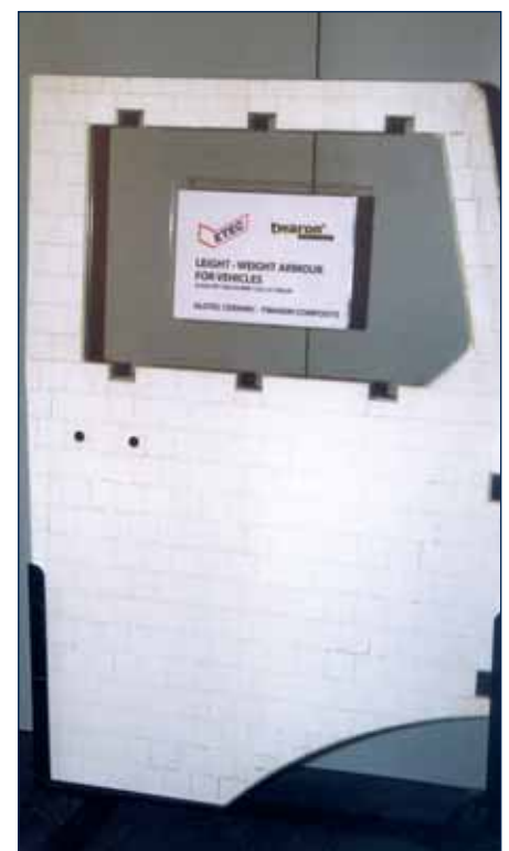
Protection panel for vehicle door UNIMOG – interior armor ALOTEC – 96 SB / Twaron composite
