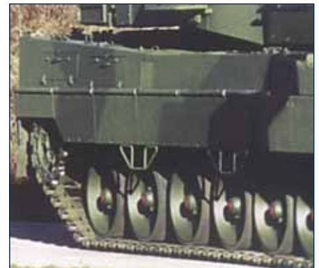
Protection for tracked vehicles/ Leopard KMW / IBD (Mexas system)
