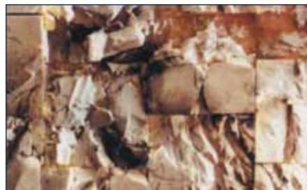
Illustration of cracked ceramic caused by fragment fire
