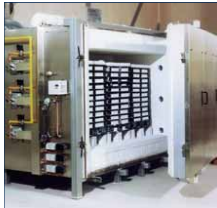
Computer-controlled high-temperature kilns ensure defined sintering processes.
