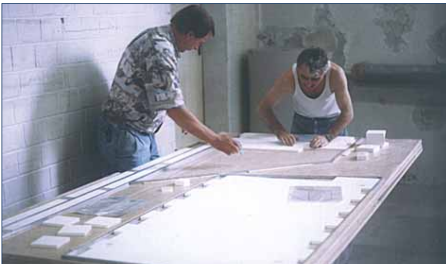
Pre-engineered and assembled ceramic have shown to be desirable at numerous projects, thus making unnecessary the expensive diamond cutting and drilling of the tiles forming the ceramic panels.
