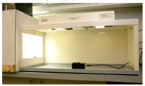
Figure 6. Daylighting controls simulator
