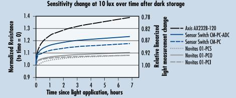
Sensitivity changes over time for several CdS cells currently used in products.
