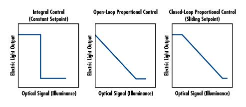
Figure 2. Archetypical response function for switching photosensor
