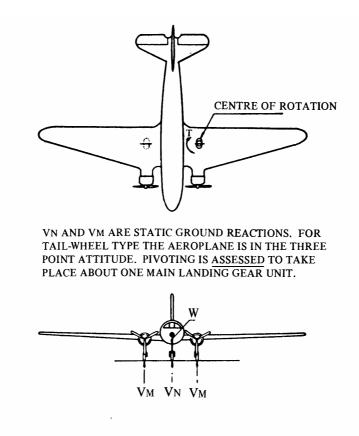
FIGURE 8 PIVOTING, NOSE- OR TAIL-WHEEL TYPE
