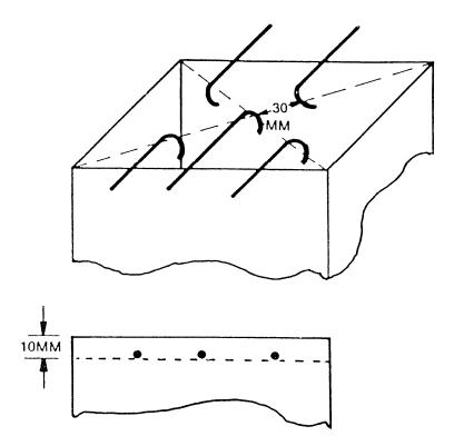
FIGURE 5. THERMOCOUPLE POSITION
