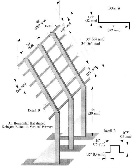
All Material 0.125" (3 mm) Thickness Except Center Vertical Former, 0.250" (6 mm) Thick
