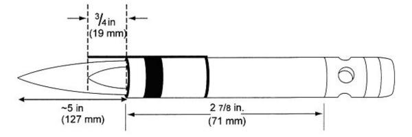
Figure 6 - Propane Pilot Burner
