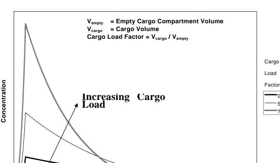
Figure 8-1. Effect of Cargo Load on Halon 1301 Concentration Levels
