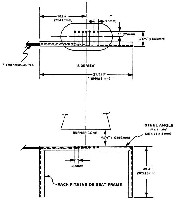
TOP VIEW THERMOCOUPLE RAKE BRACKET
