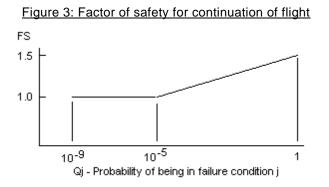
$Q_j$  = is the probability of being in the configuration with the unwanted in-flight thrust reversal  $Q_j = (T_j)(P_j)$  where:
