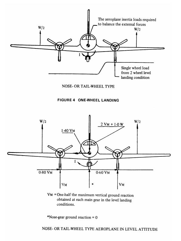
FIGURE 5 LATERAL DRIFT LANDING
