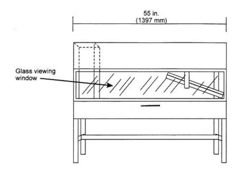
Figure 1 - Radiant Panel Test Chamber
