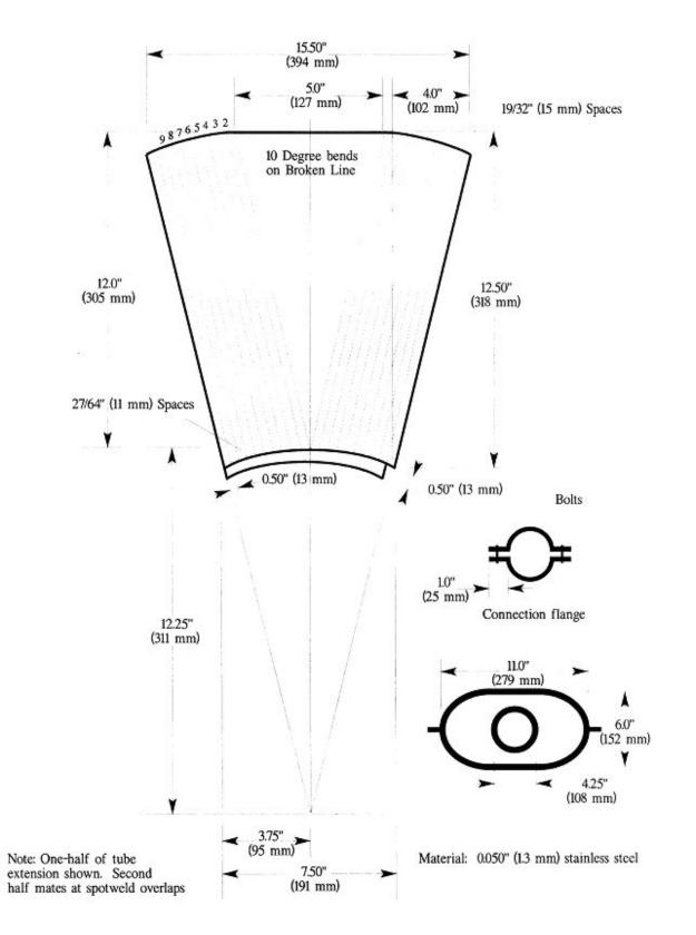
Figure 3 - Burner Draft Tube Extension Cone Diagram
