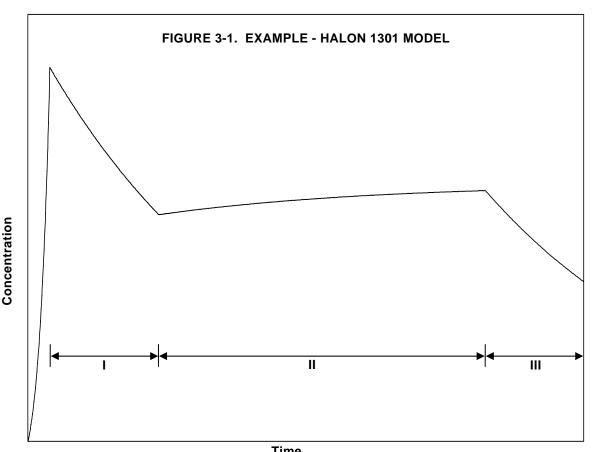
Time The second type of Halon 1301 discharge method slowly releases the fire extinguishing agent from one or more pressurised bottles into the cargo compartment. This type of discharge method is commonly known as a metering system.
