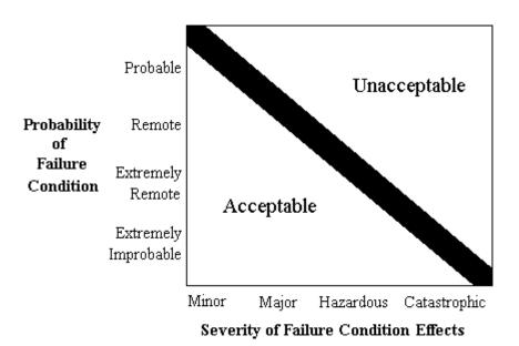
b. The safety objectives associated with Failure Conditions are described in Figure 2.
