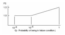
Figure 2 Factor of safety for continuation of flight
