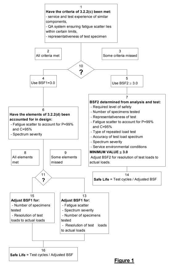
3.3 *Replacement Times.* Replacement times should be established for parts with established safe-lives and should, under CS 25.571(a)(3), be included in the information prepared under CS 25.1529. These replacement times can be extended if additional data indicates an extension is warranted. Important factors which should be considered for such extensions include, but are not limited to, the following:
