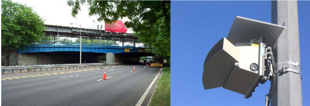
Westchester Avenue Bridge in 2001. (Credit: NYSDOT) Overheight Sensor Unit on the Hutchinson River Parkway. (Credit: Roly Parroco)
