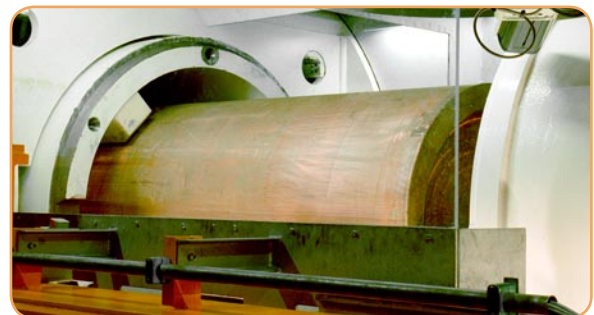
During disposal, the radiation from the canister must be screened off.
