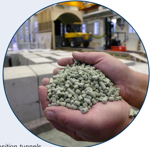
The deposition tunnels will be filled with blocks and pellets made of bentonite clay.
