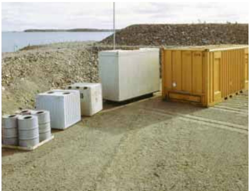
Different types of waste containers for low- and intermediate-level waste.
