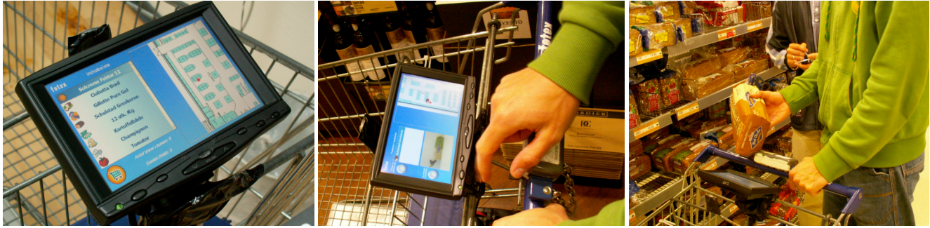
Figure 1: Illustration of CAST. The picture on the left illustrates the shopping list and the overview map of the store including the nearest product (red dot in the map). The centre picture shows a nearby product in the shopping list and its location, while the right-hand side picture illustrates the system reacting to a shopper taking a loaf of bread.
