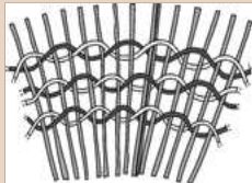
5. Scheme of braiding technique.
