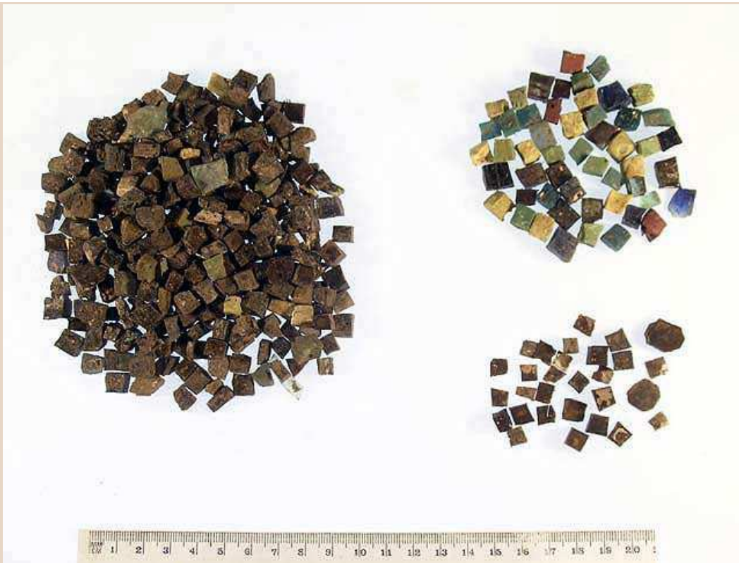
15. Glass tesserae; on left, before cleaning; on upper right, after cleaning; on lower right, gold-glass tesserae.
